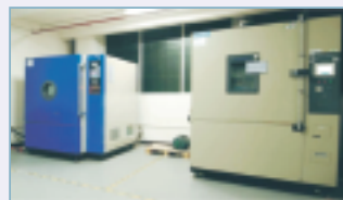
Low Prssure Test Chamber & Constant temperature and humidity test chamber
